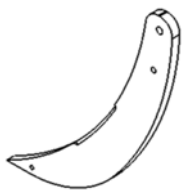
Figure 1 CAD file of the subsoiler type curved leg (type 1).
