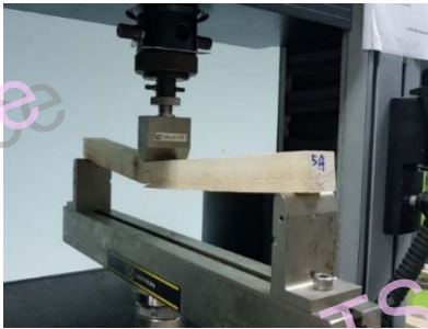
Figure 3 Testing modulus of rupture with Universal testing machine (UTM)
