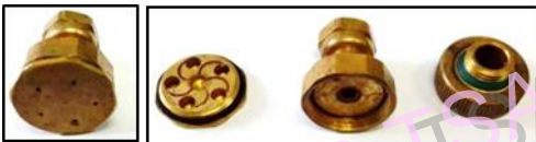
Figure 3 The hollow cone nozzle type of the spray with 5 holes
