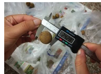
Figure 2. Measurement of the dimension of longan by using a digital caliper.
