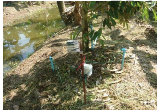
Figure 2 installation soil moisture sensor and tensiometer
