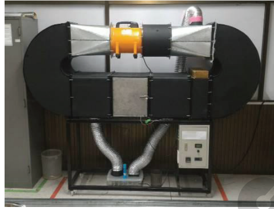
Figure 2 Closed loop hot air tunnel (laboratory scale) for drying application having air temperature controller and air velocity adjustable.
