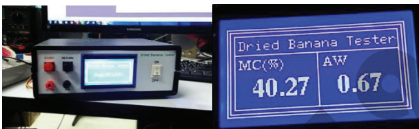
Figure 6 (a) The developed prototype moisture and aw meter of dried banana and (b) moisture content and AW on display.
