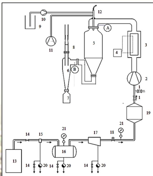
Figure 1 A schematic diagram of superheated steam spray dryer and associated units. (1) Ball valve; (2) Blower; (3) Supplementary electric heater; (4) PID controller; (5) Drying
