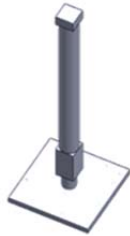
Figure 5 Hydraulic cylinder for compressing unit.
