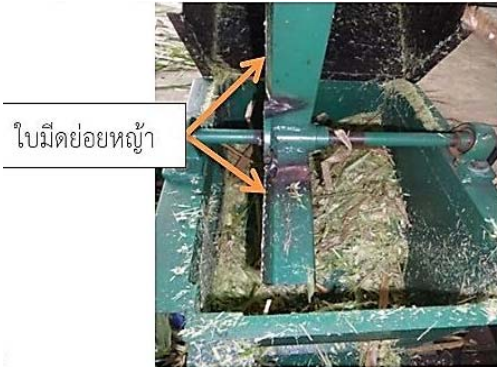
Figure 11 Closed up view of shredding unit.
