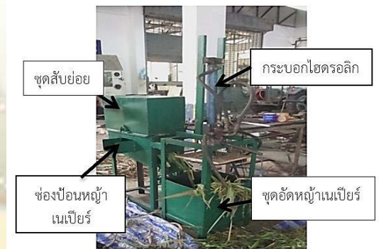
Figure 10 Testing of animal feed shredding and compressing machine.
