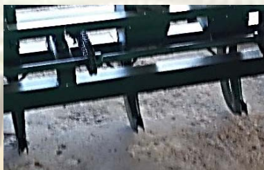
Figure 7 Covering and compacting Devices.
