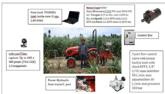
Figure 3 System details and specification of precision fertilizer machine.
