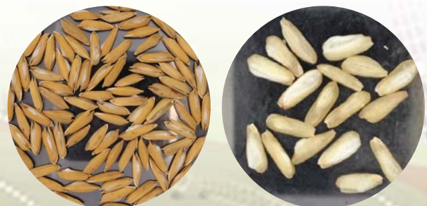
Figure 7 Soaked paddy dried by FBMW at drying air temperature of 170°C and bed depth of 5 cm (MCF = 19% d.b.).
