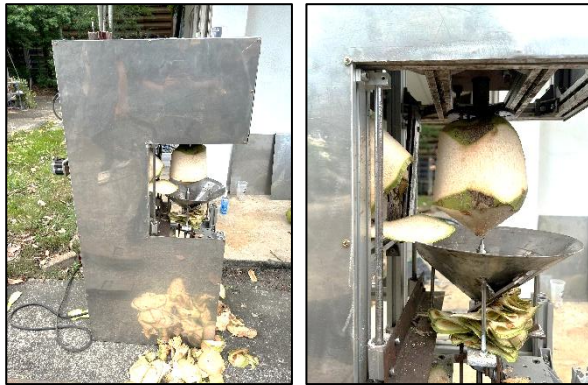
Figure 8 Automatic coconut peeling machine
