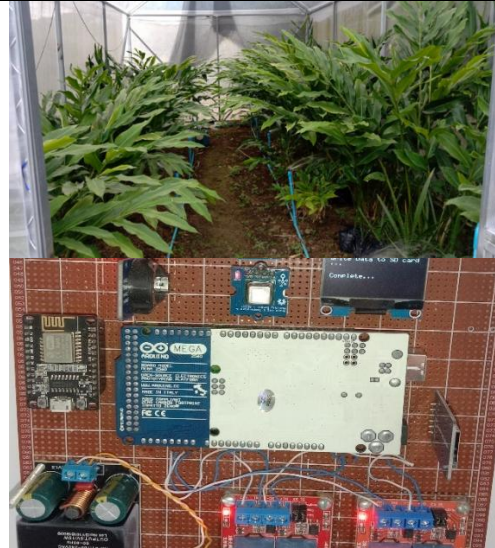
Figure 10 Cardamom is grown in an automatic greenhouse that uses data from a system that records environmental data in Thai cardamom fields by Google Apps Script combined with an embedded system.
