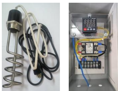
Figure 4 The heater and PID temperature control module used in the fermentation system.
