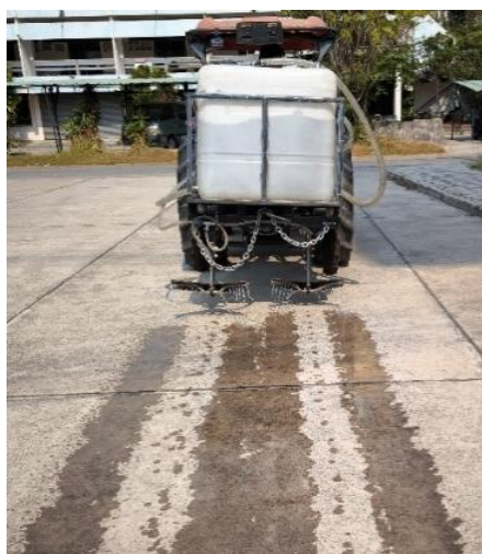
Fig. 5 Application pattern on cement floor.
