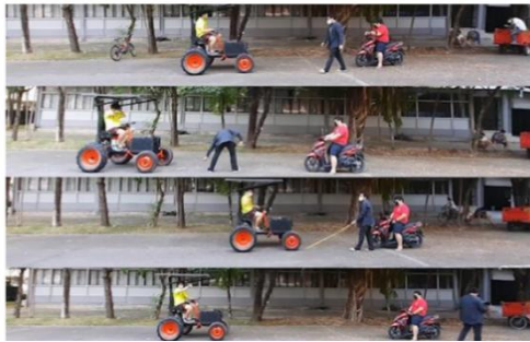
Figure 4 Images of an electric tractor driving at 5 km/h at various distances during the day.
