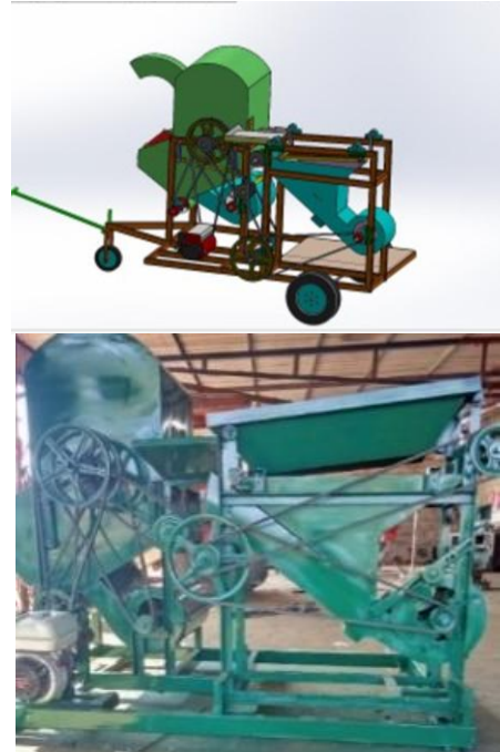
Figure 1 drawing and prototype of rice separator
