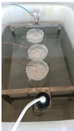
Figure 3 The developed prototype of an automated fermentation system for virgin coconut oil production.
