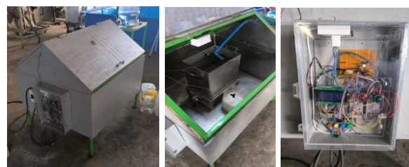
Figure 1 Experimental setup for the steam curing process
