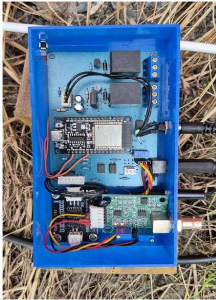
Figure 2 The ESP-32D board interfacing with the nozzle's water dispensing control circuit and TDS, pH, and temperature monitoring.
