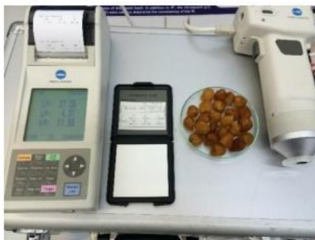
Figure 2. Photography of CR-400 chroma meter (Konica Minolta; Japan).
