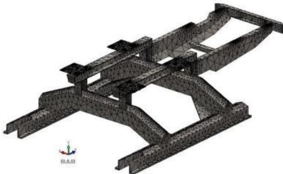
Figure 2 Mesh of the track frame model.
