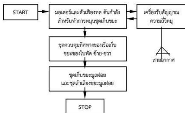
Figure 6. Created the unmanned remote control garbage collecting boat procedure.
