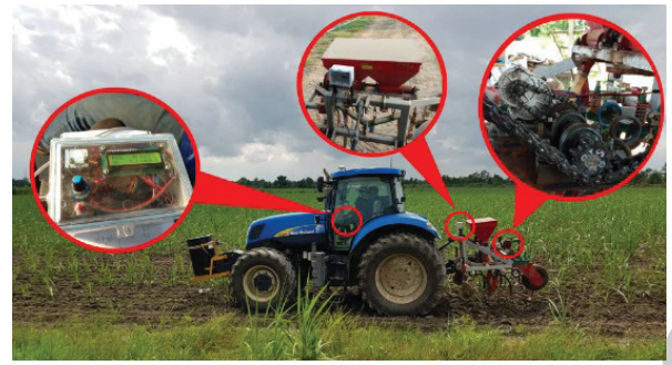
Figure 2 Installation the control system on fertilizing machine and tractor.
