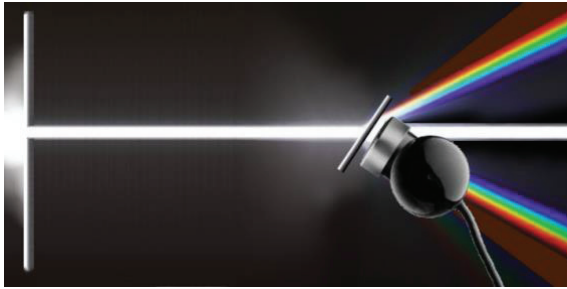
Figure 3 The refraction of light through the grating (Theremino, 2017)
