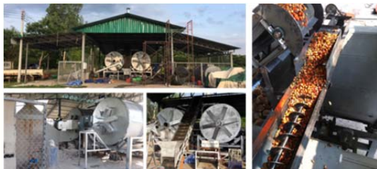
Figure 6 The rotary dryer of Palm Oil Extraction Plant.
