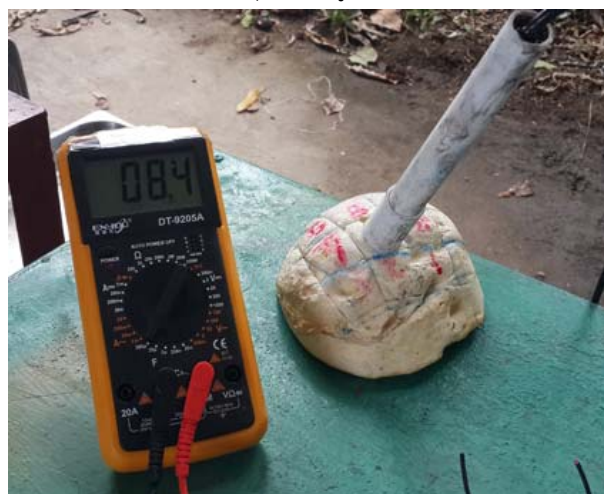
Figure 1 Investigation of electrical properties using needle-type probe.
