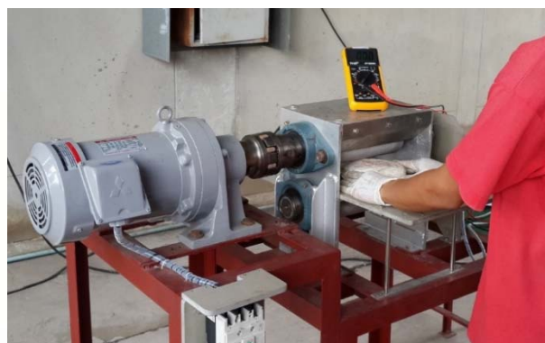
Figure 2 Investigation of electrical properties using two roller-type probe
